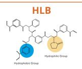
Surface area:600-800m²/g Particle size: 80-100µm Pore size: 70-90Å
