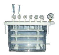
SPE vacuum manifold system process multiple samples simultaneously, saving time and effort.
